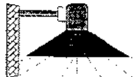
Opaque Reflector (lamp inside)
